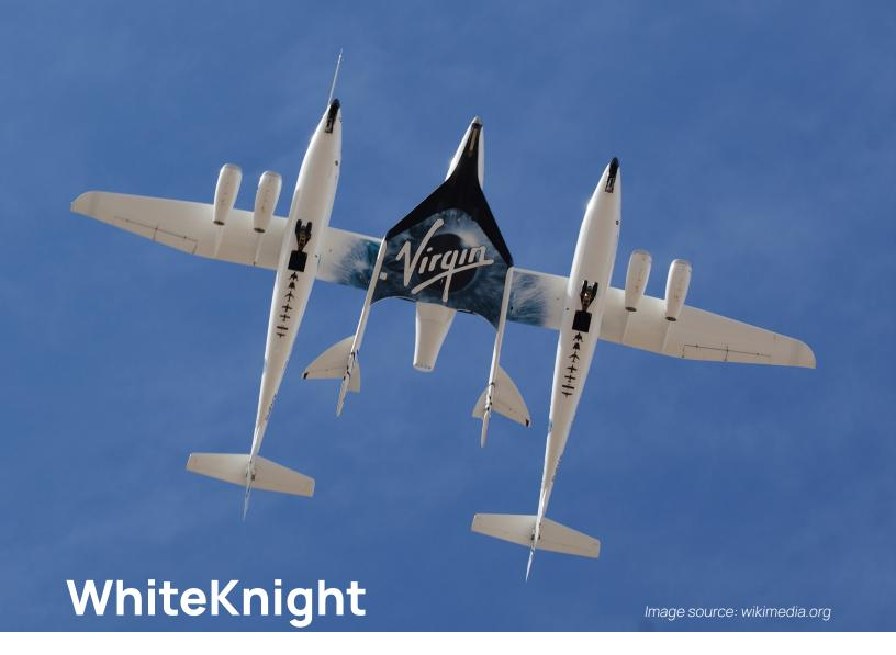
Space Composite designed a customized four-engine and duel fuselage jet aircraft known as WhiteKnight Two (WK2) to airlaunch SS2 up to an altitude of ~50,000 feet. The 140-foot main wing of WK2 houses large speed brakes that permits it to mimic SS2's aerodynamics characteristics in the gliding portions of SS2's flight. It provides an affordable, safe, and repeatable way to train Virgin Galactic's pilot for the SS2's final approach.
